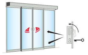
In the event of maintenance, malfunctioning or emergency, disconnect the power supply then lower the lock release lever (if installed) and manually move the door wings to their open position. To block the door wings again, bring the lock release lever back to its initial position.
